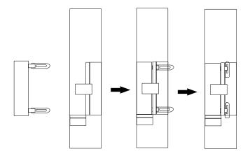
Once the outer frame is built slot the support bars into the guides to
